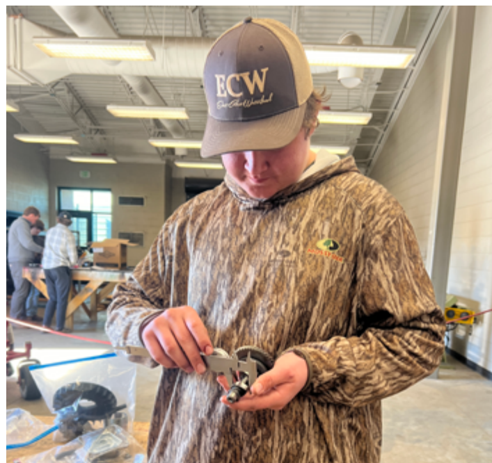
(LEFT) The students in the picture are ones who were on the 2024 Agricultural Technology and Mechanical Systems CDE team in Georgia that will compete in the national contest in October 2024. (RIGHT) A student in Agricultural Mechanics II uses a dial caliper to take the outside diameter measurements of a cam lobe to determine if the lobe has worn enough to be rejected and needs replacing.
