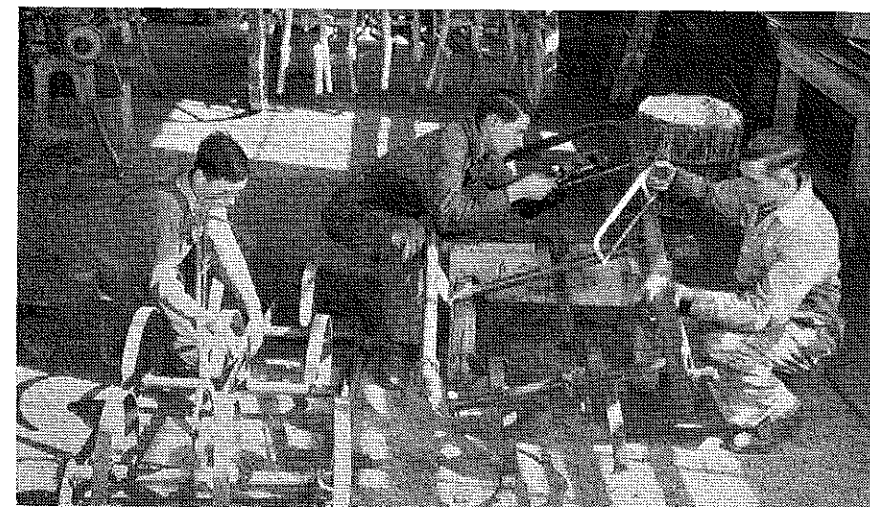
Repairing a spring-tooth harrow
