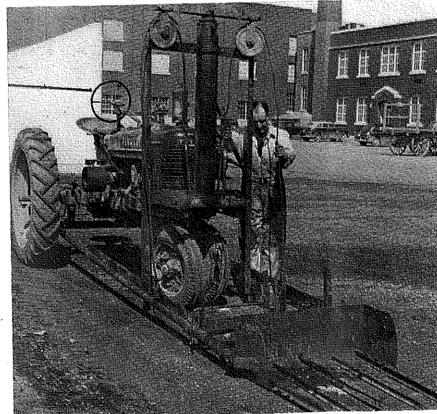
Thirty farmers in classes at Bear River have constructed 30 of these loaders during the past two years. The loader will load a spreader in three and one-half minutes. One loader keeps five men and spreaders busy so that 200 loads can be spread in one day
