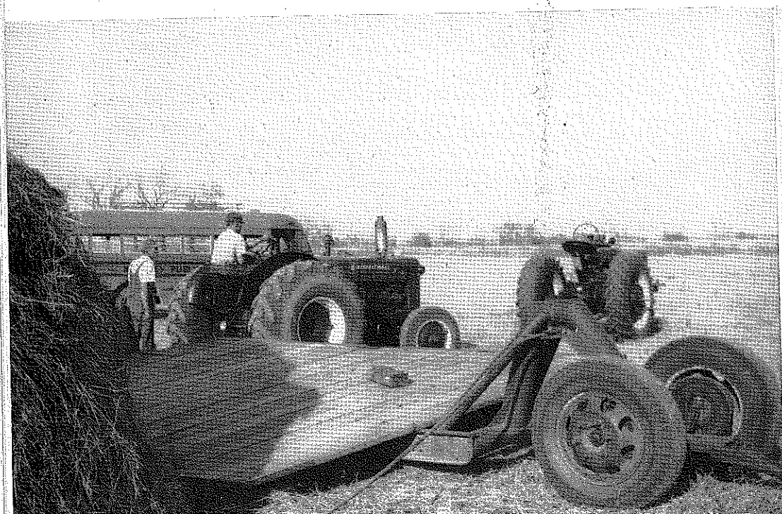
"TRACTOR TRAILER FOR HAY LOADING AND HAULING" H. W. Welton, Teacher, Kearney, Nebraska Camera: Kodak No. 1 Diomatic Film: Ansco Plenachrome 620, f.11 at 1/100
