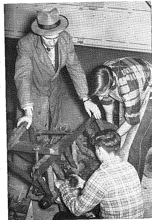
Machinery repair is rated "high" by farmers as a phase of farm mechanics. High-school boys repair a disk harrow in a school shop. —Photo by G. P. Deyoe
