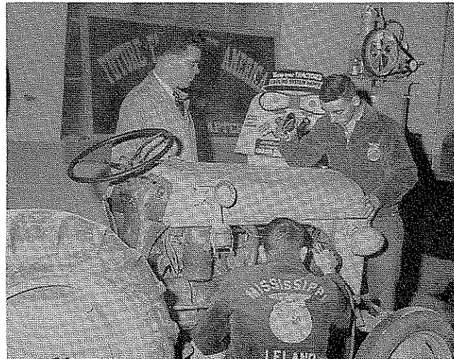
The adult program dealing with farm mechanics problems has caused greater emphasis to be placed on instruction with in-school students. Here, two members of a class in vocational agriculture, under the supervision of L. P. Jacks, Vo-Ag Instructor, are cleaning out the radiator fins and checking the water-level.
