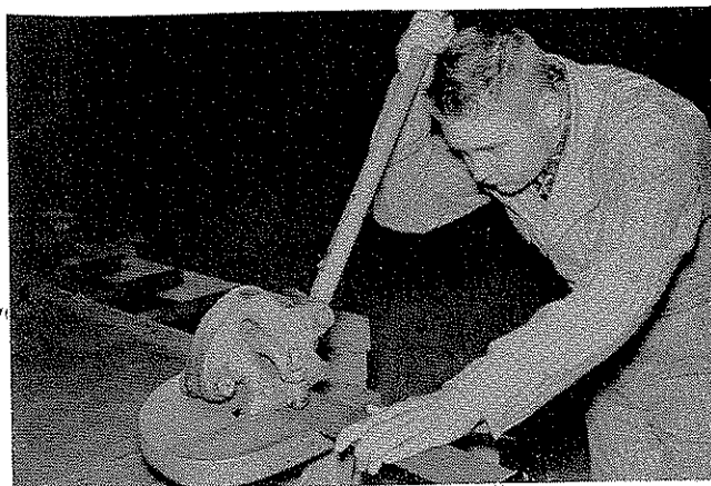
Shows student, Walter Affeldt, cutting 12 gage hot rolled strip with a B-3 Beverly Shear.
