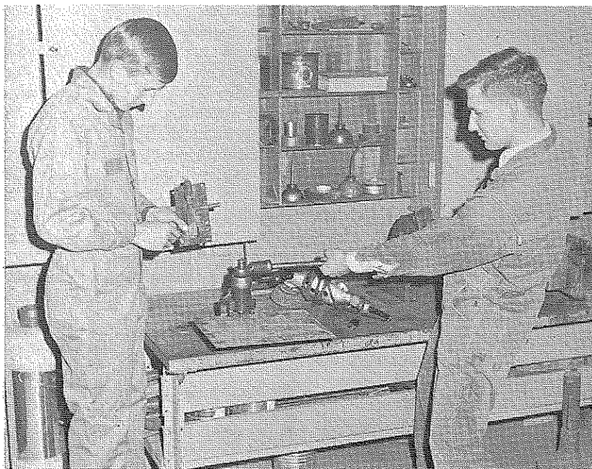
A HOLE PUNCH saves many hours of drilling and many dollars worth of bits at the Norman shop. One student punches holes in a project, while another tries a bolt in the punching job he has just completed. Holes can be punched in metal up to one-half inch thick with this device.
