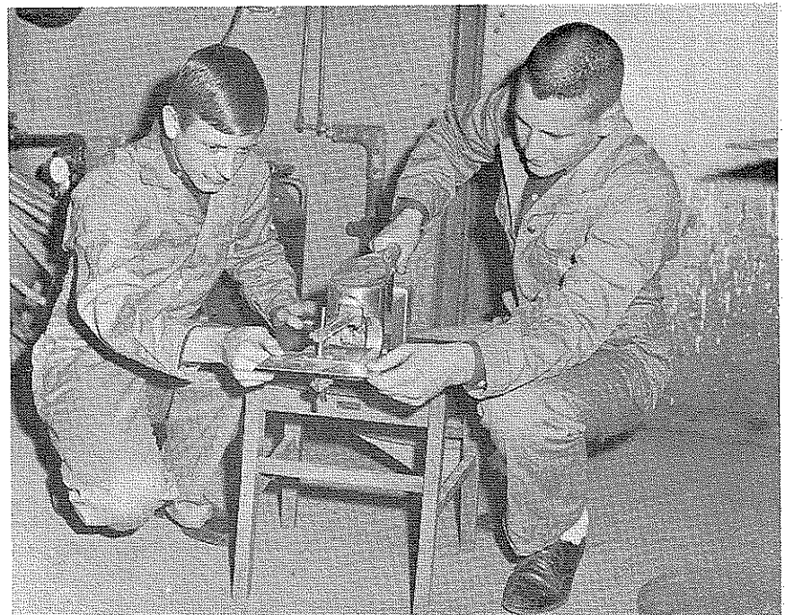
A SPOT WELDER in the Norman shop is a handy and fast way to secure sheet metals. Students use this machine on many projects requiring thinner types of metals.
