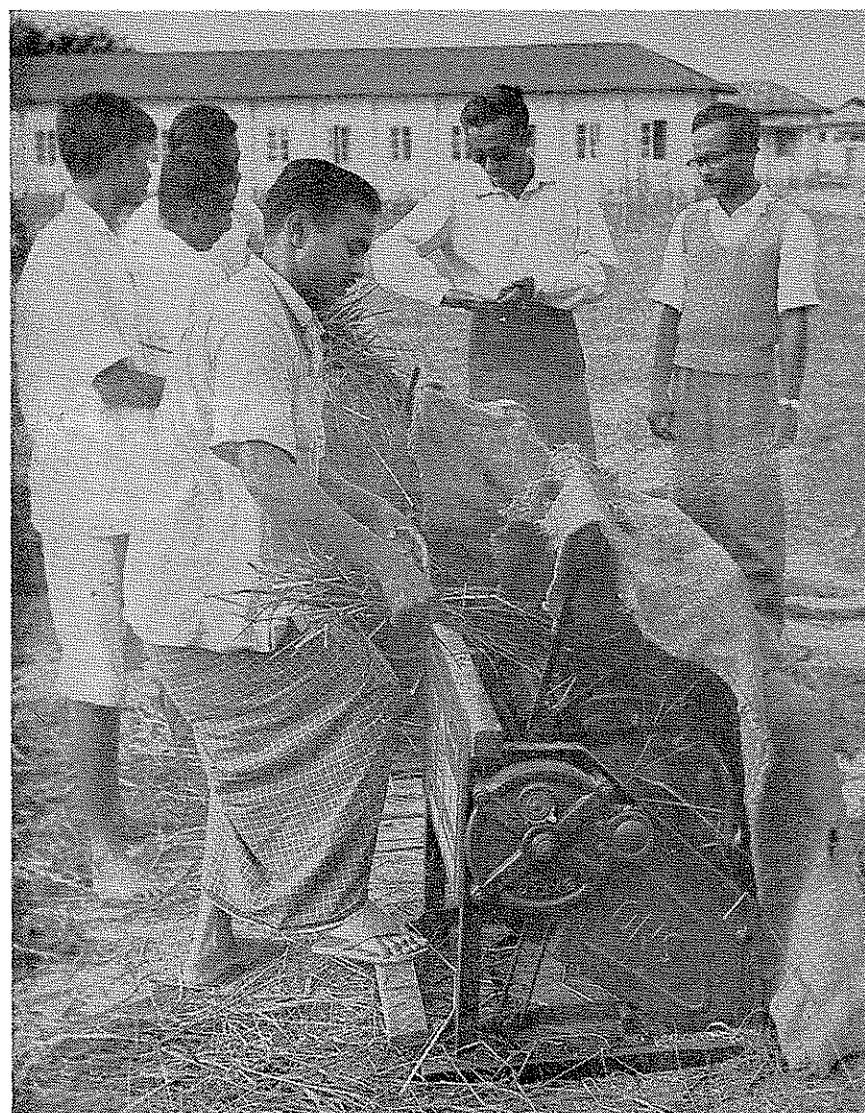
Mr. Ahmed, right, Agricultural Education Specialist in East Pakistan, and an instructor are observing the work of one-year agricultural education trainees who are learning to use Japanese-type, pedal-operated rice threshers. This method is more efficient than the use of bullocks to trample the grain. The rice was grown as a class project. Trainees also grew vegetables on individual garden plots. These men plan to organize similar projects with their high school students.
