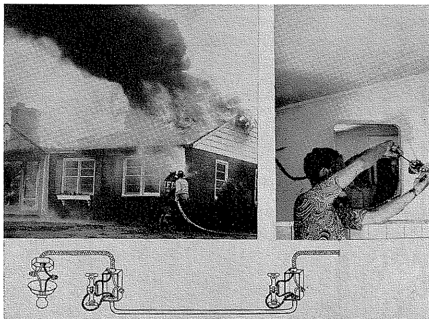
Figure 1. Expert electrical wiring, illustrated at upper right and bottom, is not enough to insure safety. The electrician must also have a thorough appreciation of the nature of electricity and its relationship to the type and size of wire. Using improper size or type of electrical wire may have caused this fire.
