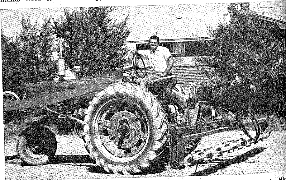
Randy Butler earned fourth award with this corrugate opener built at Minidoka County High School, Rupert, Idaho
