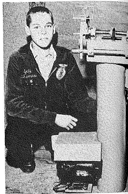
The shielded motor and belt, protective lens and tool rest of this grinder exemplifies the safety features which can be incorporated in the design and plans of a project.
