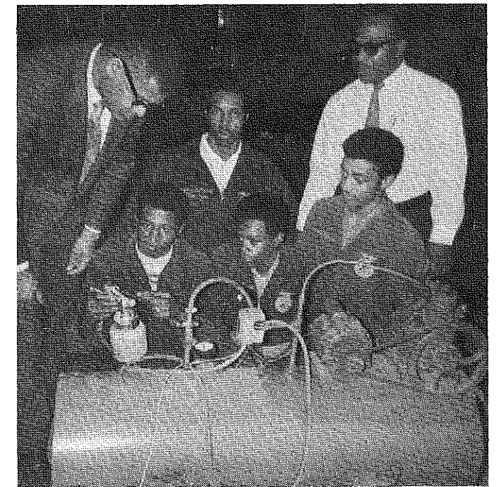
Fred Jackson, left, principal of Wesley Ray High School, Angie, Louisiana, listens to students explain the operation of a paint sprayer. The compressor unit was constructed in the agriculture department shop under the direction of Freddie Jefferson, vocational agriculture teacher. Construction materials included a discarded 40 gallon electric water tank, a one-half horsepower motor and 4 legs from a washing machine and a compressor from a refrigerator. Purchased supplies included copper tubing, pressure gauge, pressure switch, fan belt and pulley. Total cost $9.27. Approximate value $125,000. (Photo by J. C. Simmons, Area Supervisor).
