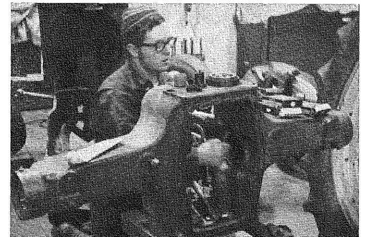
Louis Bay installing a bearing race in differential housing of a farm tractor. Tractor is literally repaired from radiator cap to drawbar pin for learning experiences.
