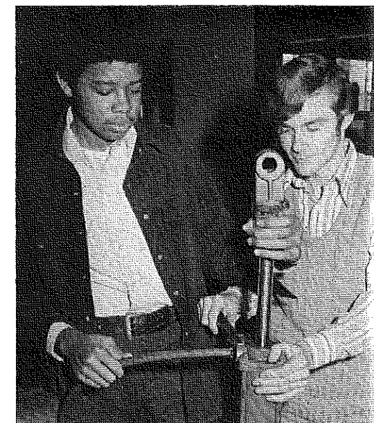
Hill and Giddens are making depth adjustments on a remote hydraulic cylinder.
