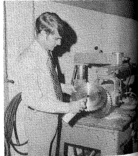
SHOP TIP—Mr. Dennis Kahl, Wood River, Nebraska, recommends household oven cleaner to remove the gum and burned-on particles from saw blades. He also recommends getting the saws sharpened before additional use. (Photo by Richard Douglass)
