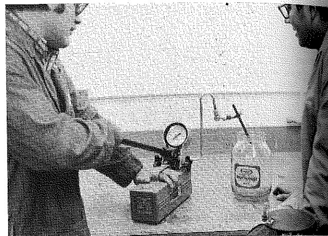
DIESEL INJECTOR TESTING — David Resch (left) and Dennis Finstad are shown testing a diesel injector in the laboratory of a diesel service and maintenance class at the University of Minnesota. This testing permits checking opening pressure, spray pattern, chatter characteristics, and return leakage. (Photo from Forrest Bear, University of Minnesota)
