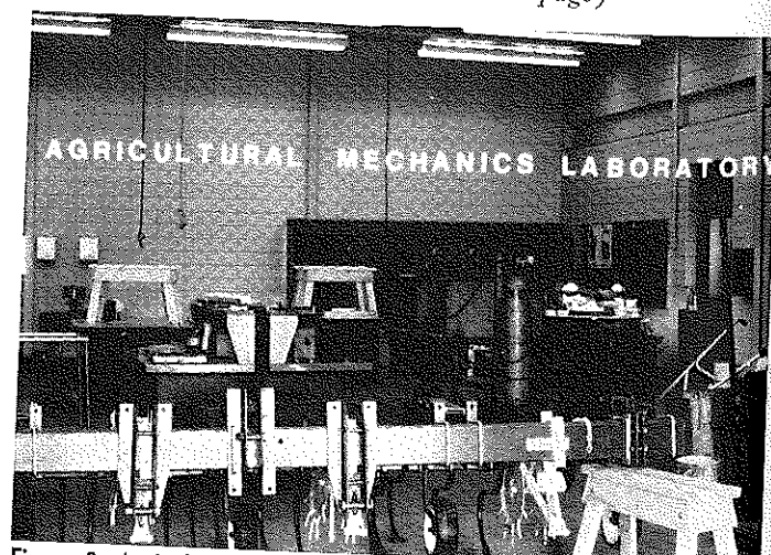
Figure 2. Agricultural Mechanics Laboratory — the facility area should be at least 3000 sq. ft. with 1700 sq. ft. of open space. The overhead door should be a minimum of 17 ft. wide and 14 ft. high to allow the entry of modern machinery.
