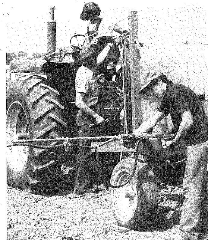
Applying a pre-emergence herbicide. Here, Thorp works with Scott Smith and Randy Seaton to double check the sprayer before applying a pre-emergence herbicide to the corn test plots at Catlin High School. The sprayer was designed and built by the agricultural machinery and welding classes, with final spacing and pump pressure calibration being done by the agricultural business management class.
