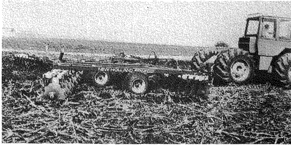
Most fields can be prepared in single pass if the tillage disk is heavy enough and properly matched to the power being used. This helps maintain an adequate ground speed, which can deliver substantial savings for farmers.
