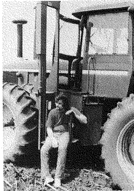
Bill Gundrum, of Royal Center, Indiana, is able to mount his John Deere 8430 tractor with the aid of a hydraulically operated manlift. Bill was paralyzed from the chest down in an automobile accident.
