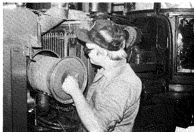
Servicing air cleaners and dust unloading valves is considered an important skill of the "set-up mechanic".
