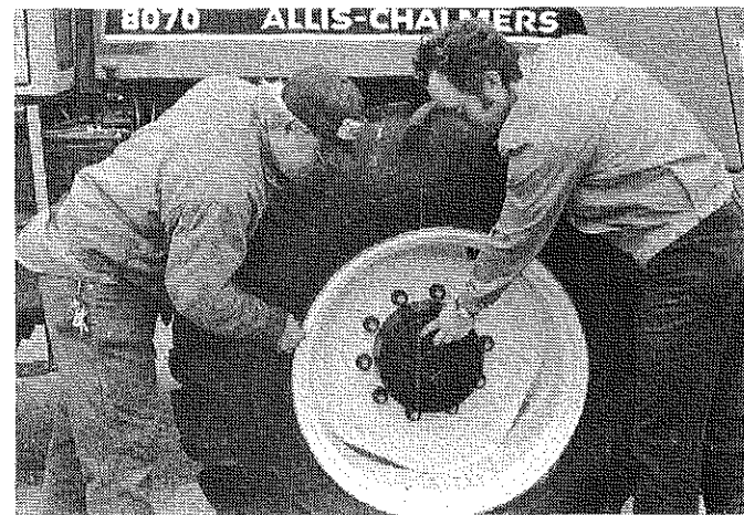
Student and manager discuss checking the oil level in the mechanical front wheel drive on a tractor.
