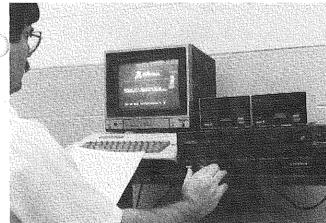
Using an interface device, you can combine the basic function of a videodisc player or VCR, the storage and playback of video images, with the interactive capabilities of a computer, all in one interactive program. (Photograph courtesy of Jim Wren, AAVIM.)
